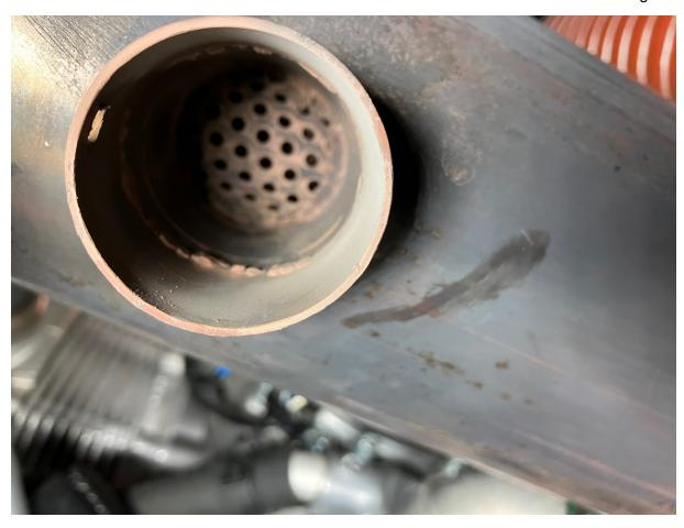
This image depicts the restriction. Note how you can see the exterior curvature of the perforated tubing.
