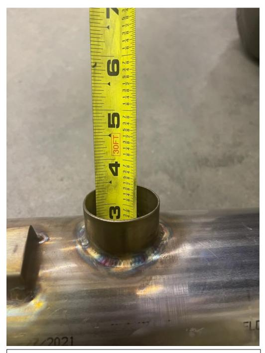
This measurement depicts the depth of the perforated tubing on a correct installation.
