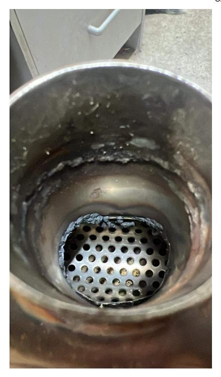
This is an image of a muffler that is correct. Note how the perforated tubing is cut away where the exit pipe joins the perforated tube.
