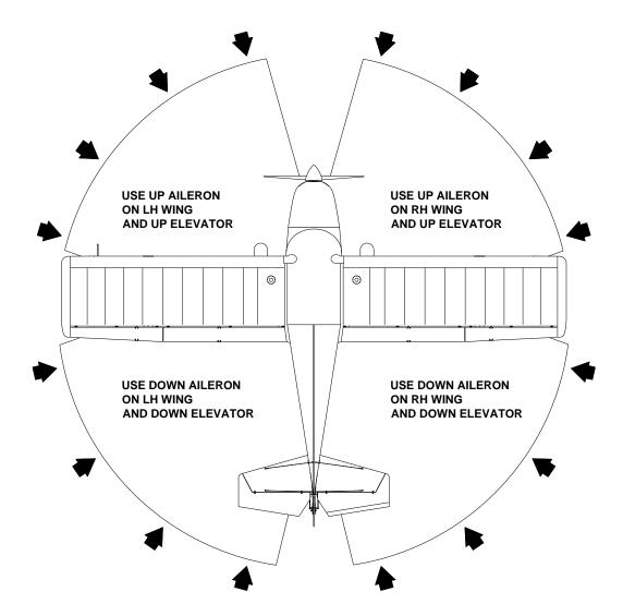
The arrows identify the wind direction. It is very important to hold the controls as described, even when the aircraft is not moving.
