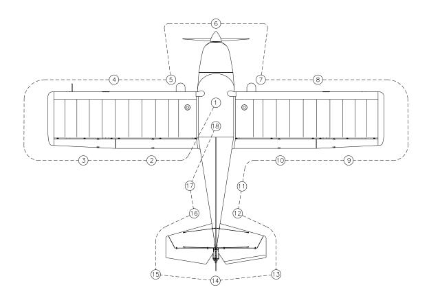
**The entire outer surface** of the aircraft should be inspected for damage of any kind during the pre-flight inspection. This is especially important due the fact that the aircraft is fabric covered.
