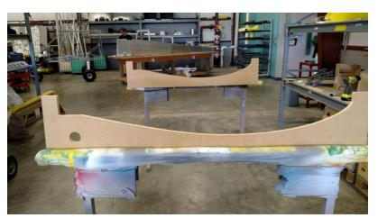
kit. To assure accurate wing twist we provide machined out supports of composite wood. Attach the jigs to the saw horses with the bottom edge of the supports level with the world. The sawhorses should be on level ground and set apart the distance between the wing root and strut attach point. The wing is then clamped or taped into
