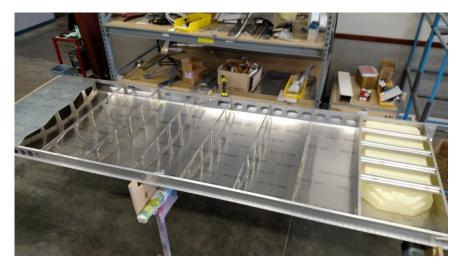
the jigs, ready for installation of the bottom panel. Ok, so you may ask, how are the wings assembled up to this point? It is done on the same two sawhorses, only minus the jigs. The goal is to provide a kit with all the tricks built in for extra fast and accurate assembly, and yet still be within the FAA's 51% ruling for EAB.
