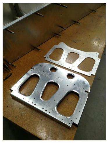
Updated Station 8 bulkhead: Station 8 has been revised to be lighter and stronger to take the tail wheel loads. We get such a nice clean cut that you won't, in general, have to remove burrs or do any edge sanding. This really speeds assembly. We should be seeing a completed tailcone for load testing before long.
