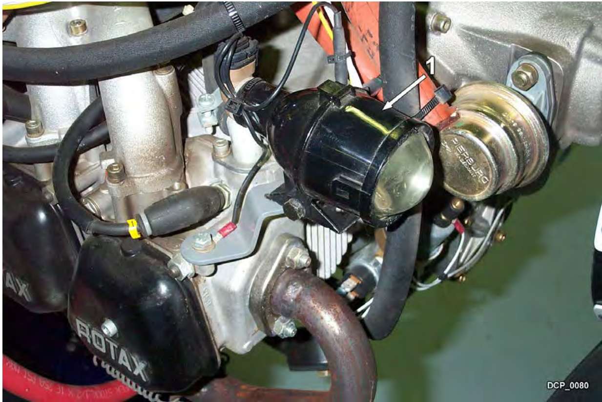
1. ECONO LANDING LIGHT FROM WAL-MART, BLAZER PROJECTOR BEAM FOG LAMP SYSTEM (C4072K)
