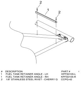
FIGURE 1 - Parts required for Installation
