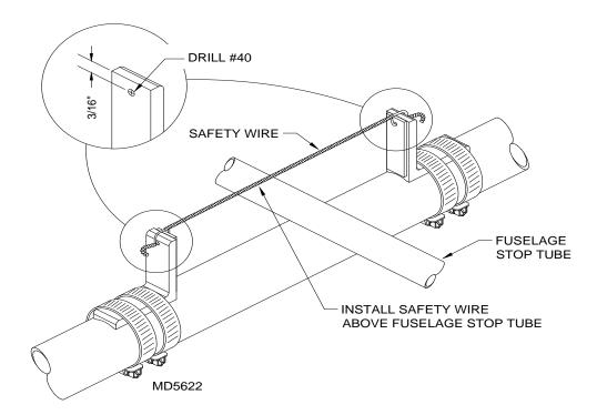
FIGURE 1 - Modification of Pitch Stops and installation of Safety Wire
