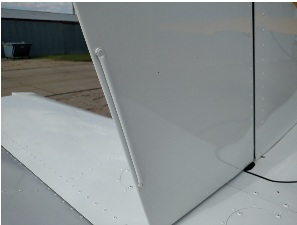
Permanent bump trim using 1/4" Aluminum tubing.
